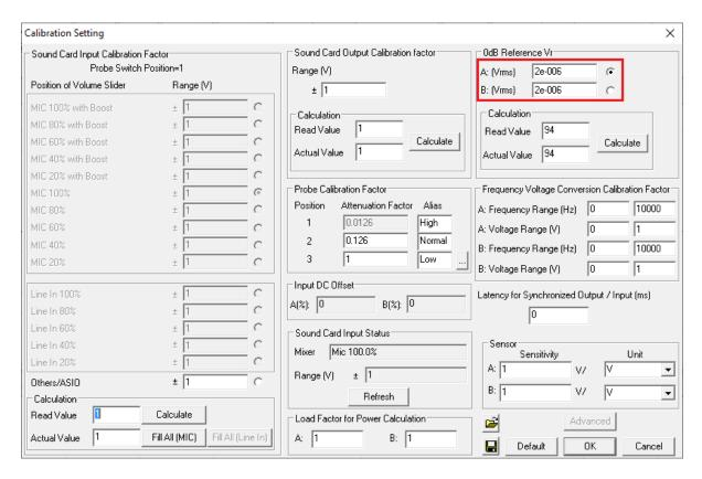
It is possible to calibrate the sound level yourself using a sound level calibrator or a sound level meter. Please refer to Section 2.6.2.3.5 of the Multi-Instrument software manual for details.
