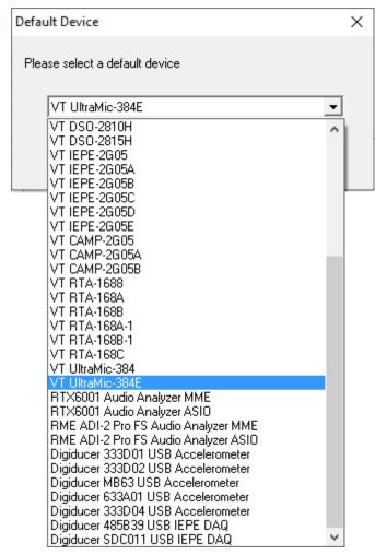
All sound cards in the system will be listed as Sound Card MME devices. To select VT UltraMic-384E for data acquisition, with the VT UltraMic-384E connected, go to [Setting]>[ADC Device], and make sure that Sound Card MME is selected in the Device Model selection box, and select UltraMic384E in the Device No. selection box, as shown below.
